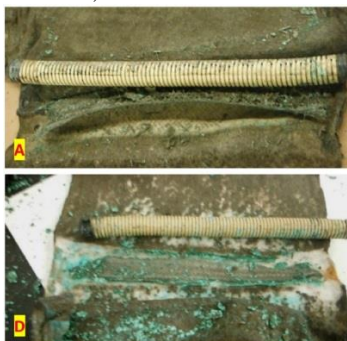
Fig. 3: The condition of the anodes at the end of the experiments A and D[83].
